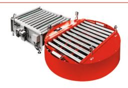
The TURNTABLE STATION and ROLLER/CHAIN EXCHANGER enable the palletized loads to change direction. The turntable station consists of a roller conveyors or chain conveyors able to rotate on its axis allowing the 90° exit of the palletized loads without changing the pallet orientation in the transport direction.
