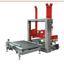
The EMPTY PALLET DISPENSER satisfies on one side the requirement of depositing empty pallets and on the other feeding pallets for the production line. The operator will deposit empty pallets in the warehouse and the automatic device, equipped with conveyors, will dispense the pallets to the production line. The capacity of the system is up to 12 pallets.
