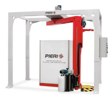
SILVER WAVE is PIERI's semi-automatic arm machine. SILVER WAVE is a stand-alone system and it represents the perfect solution for pallets with unstable loads. The loading will be inside the machine with the forklift or pallet truck. The operator will start the automatic wrapping cycle with a remote control.
