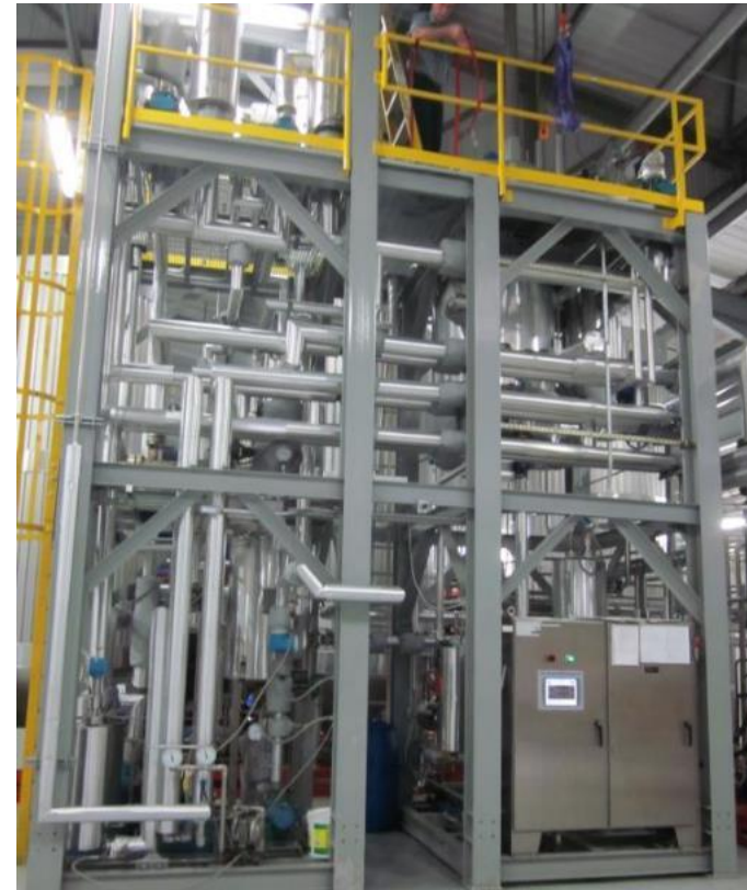
Wiped Film Evaporator Systems: Complete modular process systems, pre-assembled and tested
