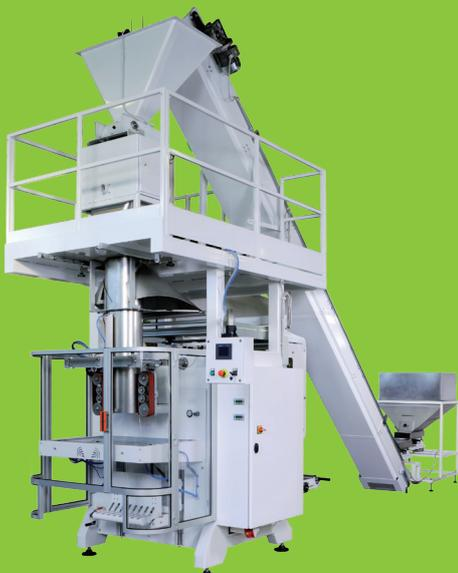
**Loading hopper + Elevator belt + Weighing unit + TITAN 50**
